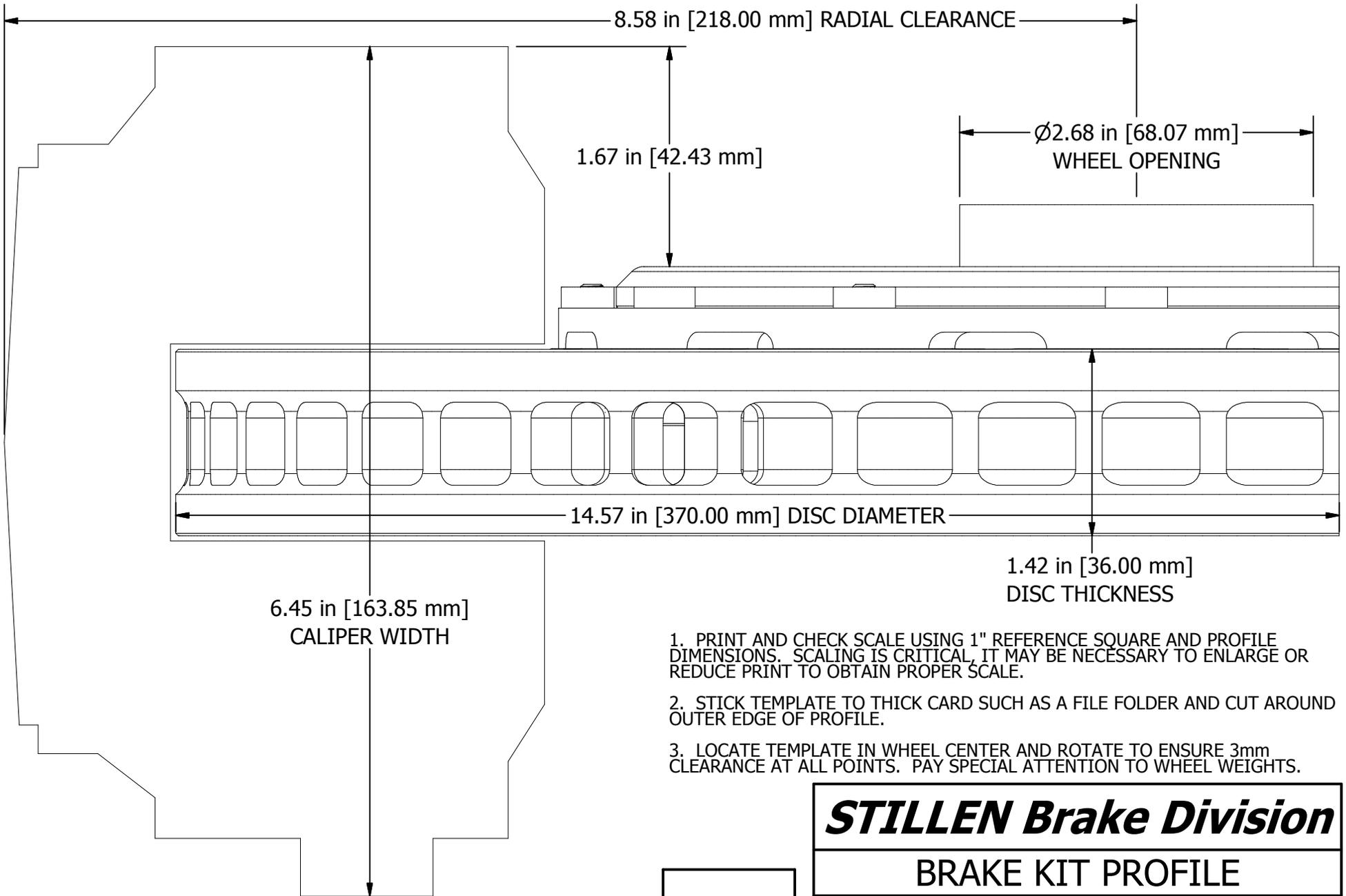
1. PRINT AND CHECK SCALE USING 1" REFERENCE SQUARE AND PROFILE DIMENSIONS. SCALING IS CRITICAL, IT MAY BE NECESSARY TO ENLARGE OR REDUCE PRINT TO OBTAIN PROPER SCALE.
